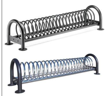
Bike support made up of a spiral-shaped rack in tube Ø22mm welded to two horizontal steel tubes Ø48 mm. At the extremities of the two horizontal tubulars drilled brackets are welded to be then fixed to lateral arched supports. The two arches are made in Ø60 tube and are provided with 4 welded plates Ø150 for ground anchoring with bolts.
