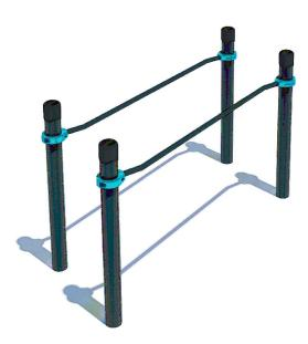
The complex consists of four vertical columns and two parallel bars 1790mm in length. The distance between the parallel bars is 716 mm. Construction is secured together with siluminium clamps.
