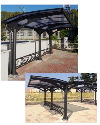
Larus Bike is a modular cover composed of two lateral supports in steel tubular Ø 121MM (which can arrive up to 152 mm for bigger bespoke covers) and of 8-mm-thick steel sheet sides, which are duly bent and laser-cut.
