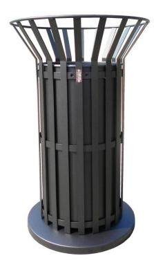
Litter bin composed by 20 stripes in steel plate 25x4 mm welded vertically all along the container to three horizontal rings in steel plate 25x4 mm and on the top properly folded and welded to a ring in steel rod  $\emptyset$  10 mm.
