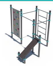
The complex consists of eight vertical columns of different height, three crossbars 500 mm in length, three crossbars 1200 mm in length, Swedish wall, climbing wall and a composite material bench for abs. Height of the Swedish wall - 2073 mm. The distance between the crossbars of the Swedish wall - 407 mm. Height of the climbing wall - 2073 mm. Construction is secured together with siluminium clamps. Weight 339,3 kg
