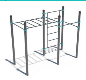
The complex consists of six vertical columns, two crossbars 1200 mm in length, Swedish wall and a classic monkey bar. Height of the Swedish wall - 2073 mm, width - 1200 mm. The distance between the crossbars of the Swedish wall - 407 mm. The length of monkey bars is 1900 mm. The distance between the crossbars of the monkey bar is 311 mm. Construction is secured together with siluminium clamps. Weight- 293,9 kg.
