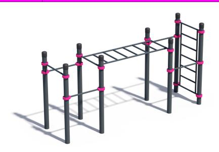
The complex consists of eight vertical columns, five crossbars 800 mm in length, a horizontal monkey bar and a Swedish wall. Length of the monkey bar is 1952 mm, width – 800 mm, distance between each crossbar is 274 mm. Height of the Swedish wall is 1678 mm, width – 800 mm, distance between each crossbar is 274 mm. The complex is secured together with aluminium clamps.
