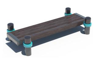
The construction consists of four vertical columns and composite material bench with the length of 1500 mm, width of 400 mm. The distance between the columns is 598 mm. The standard height of the bench is 425 mm. Construction is secured together with siluminium clamps. Weight- 79,0 kg.
