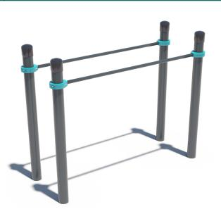
The construction consists of four vertical columns and two horizontal crossbars. Crossbar length is 1758 mm. The distance between the parallel bars is 600 mm. Crossbars are secured to the columns with siluminium clamps at the height of 1300 mm from the foundation. Weight 96,2 kg.
