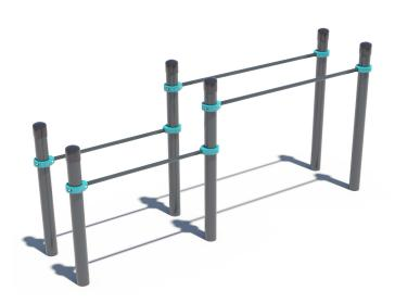
The construction consists of six vertical columns of different height and four horizontal crossbars: 2 pieces – 1200 mm in length, 2 pieces – 1758 mm in length. Crossbars are placed parallel. The distance between the parallel bars is 600 mm. Construction is secured together with siluminium clamps. Weight 138,2 kg
