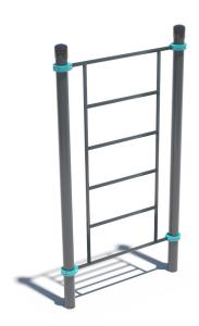
The construction consists of two vertical columns and Swedish wall with height of 2073 mm. Swedish wall consist of crossbars. The distance between the crossbars is 407 mm. The width of the Swedish wall is 1200 mm. Construction is secured together with siluminium clamps. Weight 103.2 kg
