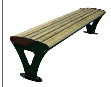
Bench with a metal structure made up of 2 supports in laser-cut steel sheet 8 mm thick and welded on an elliptical base plate 300x100 th.8mm for the surface fixing with bolts.
