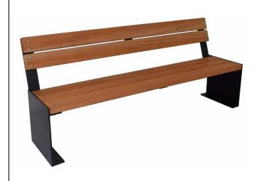
Bench Amburgo with backrest has a structure in galvanized and powder coated steel, composed by two supports in laser-cut steel sheet 8 mm thick, to which are welded drilled base plates for the anchoring to the ground with bolts.
