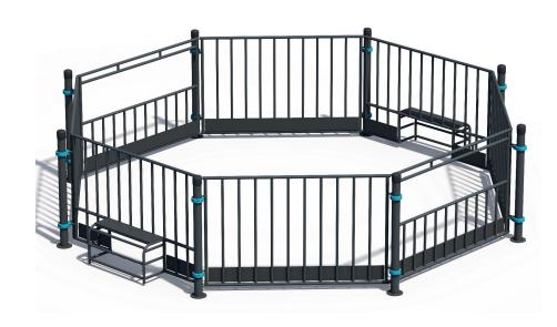
The structure consists of eight vertical columns 1600 mm in height and eight sections with vertical crossbars. Height of each section is 1500 mm, length - 2381 mm. The structure is secured together using siluminium clamps.
